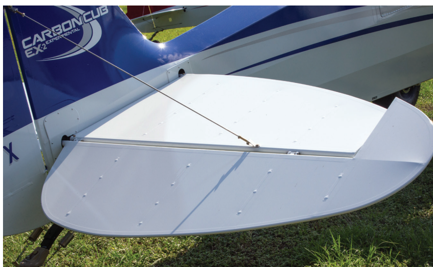
G-Series control surfaces feature adjustable elevator stops for improved pitch stability and aerodynamic flaps with repositioned pivot arms for enhanced low speed handling.
